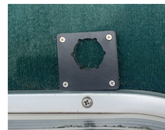
2. Bottom plate once fastened to the deck
