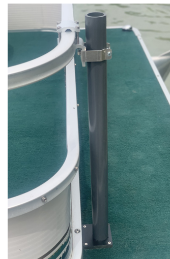
1. Full view of bracket mounted to Pontoon Boat
